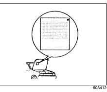
The EPA emission compliance label is located under the hood. It provides much of the information needed to perform an engine tune-up on your vehicle.
